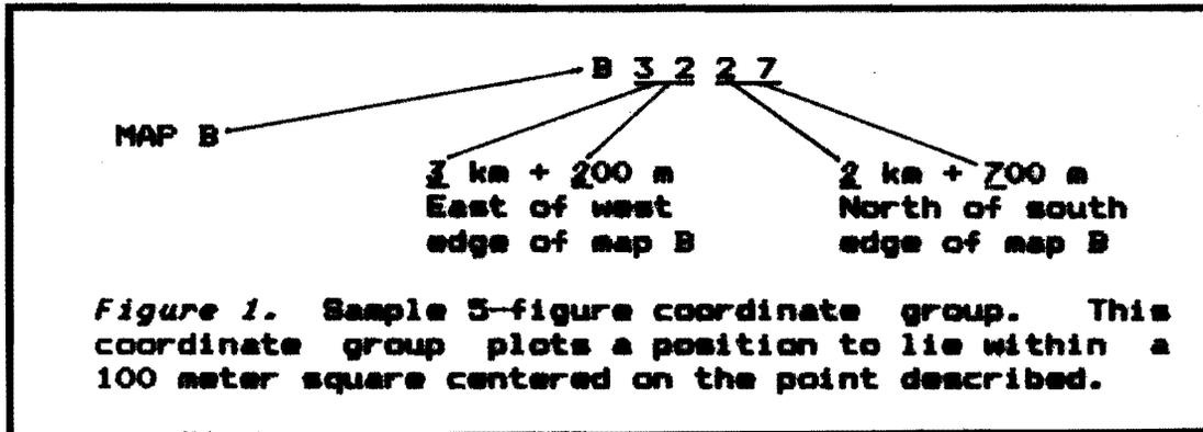
It should be noted that any position within the 100 meter square will be described by the coordinate group B3227. Consequently the maximum error will be 70 meters. To specify the position to within a 10 meter square (which is only 0.42 x 0.42 mm on the map!), the coordinates can be taken to seven figures as shown in figure 2.
