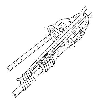
An illustration of the prusik minding pulley. Note that the grapevine knots do not have to be placed on top of the prusick knot; this was done for simplicity in the drawing.
