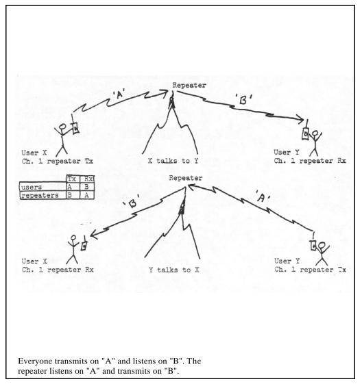
A repeater listens on frequency "A" (the *input*) and retransmits what it hears on frequency "B" (the *output*). Repeater users transmit on "A" (the repeater input) and listen on "B" (the repeater output). This system is often called "duplex" operation, as two frequencies are used to pass traffic.
